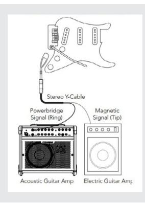
Plug a stereo "Y" cable into the output of the Hybrid and split the magnetic and piezo pickup signals to separate destinations. You will need a stereo "Y" cable that has one stereo male 1/4" plug to two mono 1/4" plugs. Send the piezo signal (Ring) to any instrument level audio input, such as an acoustic instrument amplifier or PA system. Send the magnetic pickup signal (Tip) to a traditional electric guitar amplifier.
