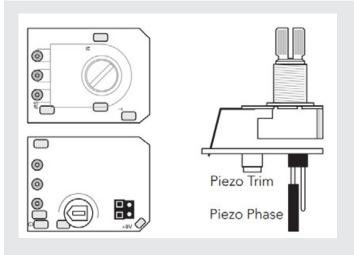
The Fishman Powerchip can be found by removing the control cover on the lower back of the your Hybrid. Adjust the small rotary trim pot on the backside of the Powerchip to match piezo and magnetic pickup levels. Move the Phase jumper on the backside of the Powerchip to eliminate phase cancellation between the piezo and magnetic pickups.
